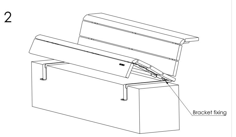
Assemble seat by sliding into bracket fixing at an angle
